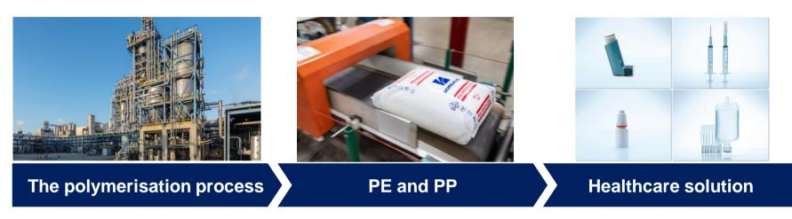
Polymerisation is a chemical reaction caused by a catalyst (for PP and HDPE) where monomer purity is key for a continuous process in this closed environment Bormed<sup>™</sup> PE and PP polymers: dedicated to the healthcare industry and delivered to converters / CDMOs, usually as 2-to-3-millimetre particles (pellets)
