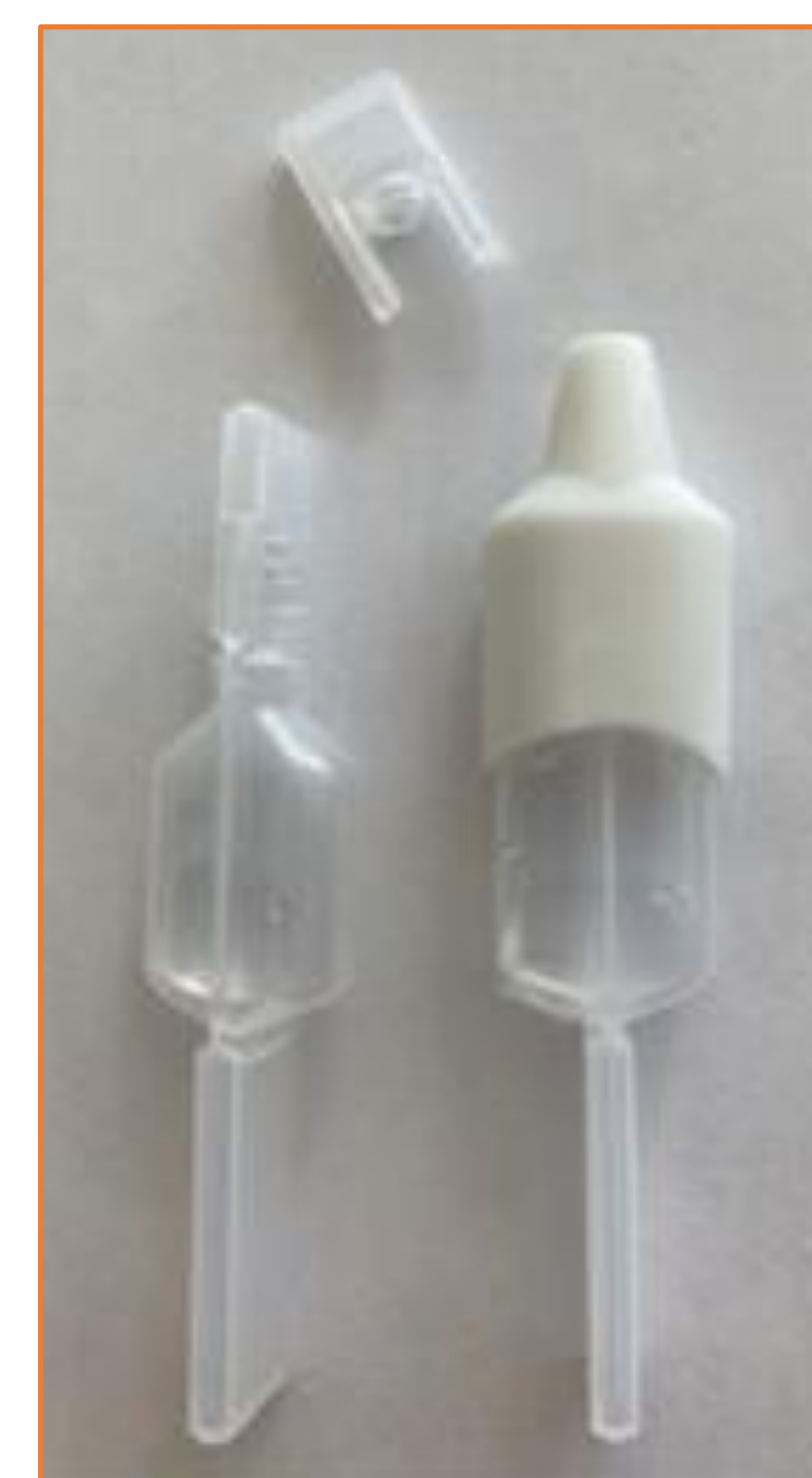
Figure 1: Illustration of Euroject® BFS container and prototype swirl-chamber based spray nozzles.
