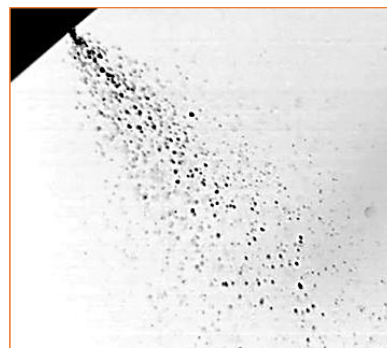
Figure 5 : High speed imaging of the Euroject® BFS nasal spray.
