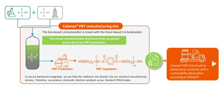
We can feed the bio 1,4 Butanediol and mix directly into our standard manufacturing process. This allows Celanese to offer our customers Celanex® PBT ECO-B as the sustainable version of most of our Celanex® PBT grades.
