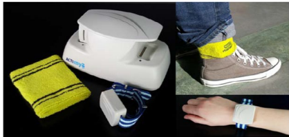
Figure 1. Main components (A), the wearable device and system attached to ankle (B) and to the wrist (C)
